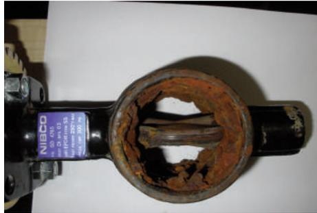
A build-up of limescale from untreated hard water can quickly cause water heaters and valves to fail
