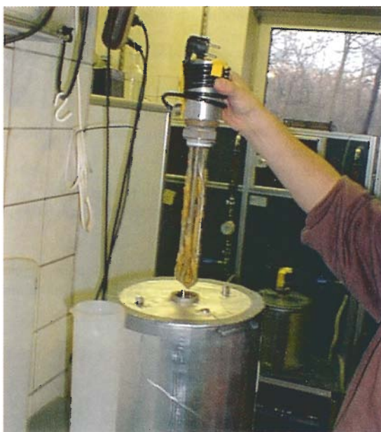
Removing the heater coil from one of the water heaters of the W512 test rig
