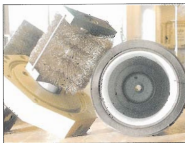
Bottom. Detail of bowl, brush, stanchion and armature. The Titanium mesh is held in place by the white liner.
